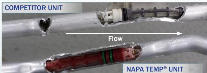
Competitor orifice tube installed backwards, preventing it from filtering debris properly.
