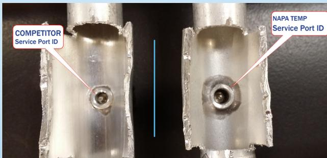
Competitor service port inner diameter is smaller than the NAPA Temp® unit, increasing system charge time.
