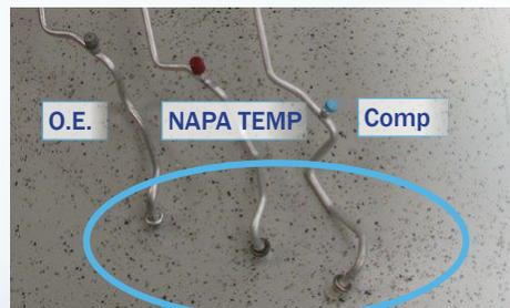
Competitor design does not match the O.E. line design causing the installer to torque the fitting to the condenser, creating stress to the line.
