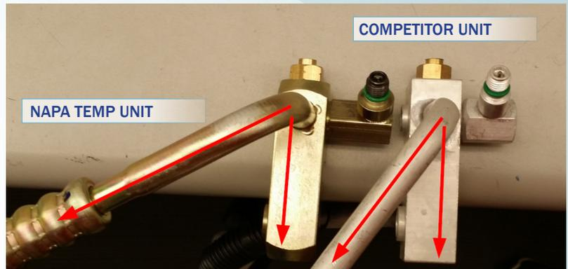
Competitor incorrect angle from the manifold block will cause installer to manipulate line in order to install.
