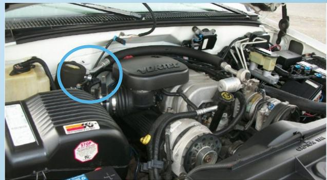
Competitor unit has wrong bend leading to the accumulator. This forces the installer to twist and manipulate the line in order to install on the vehicle, which may cause damage and stress to hose and crimps.
