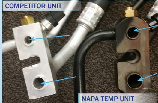
Competitors manifold inner diameter is smaller than the NAPA Temp® and the O.E. unit, restricting oil and refrigerant flow.
