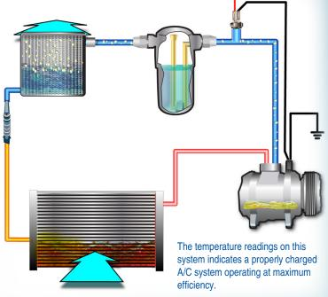
In an HVAC system the refrigerant changes state at the evaporator and at the condenser.
