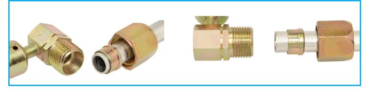
The fitting that uses an o-ring uses a shorter brass ferrule. The taper of the ferrule goes into the nut so that the flat portion of the shoulder fits against the o-ring as it fits into a groove in the fitting. Do not install the o-ring until the ferrule has been set. The ferrule must be set in place on the tube in the same manner as the steel ferrule. Install the o-ring, tightening as you would any o-ring fitting and leak test.
