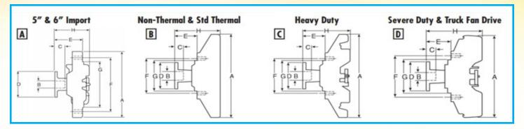
When disengaged, a fan clutch is designed to operate at 20 to 30 percent of the driven speed to help reduce the parasitic drain on the engine, increasing fuel economy. One of the primary differences between a Standard Duty, Heavy Duty, and Severe Duty fan clutch is the driven fan speed when engaged.
