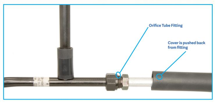
The fitting is covered with a protective rubber cover. The cover makes it hard to see the fitting and that the orifice tube is replaceable.
