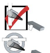
**ADVANTAGE**— Contact is not necessary, making it easier to take readings in hard to reach locations. Best results occur when readings are taken within two inches and inline with the component.
