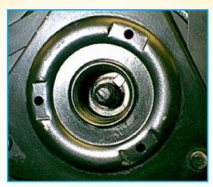
Should you receive a Delphi Harrison (GM) type compressor without the shaft nut, **DO NOT** attempt to install one. Attempting to install a nut on the shaft could alter the compressor clutch air gap.
