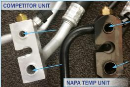
Competitors manifold inner diameter is smaller than the NAPA Temp® and the O.E. unit, restricting oil and refrigerant flow.
