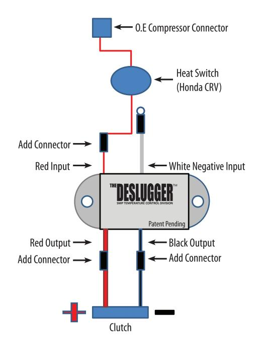
Note: Deslugger functions by pulsating clutch ground circuit during initial compressor engagement.
