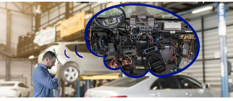
Tearing the dash apart to replace the heater core is a time-consuming repair. To ensure that your customers only do the job once, NAPA® Temp Heater Cores are leak, pressure, and vibration tested for trouble-free performance.
