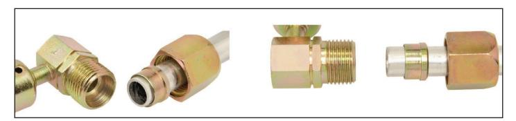
The fitting that uses an o-ring uses a shorter brass ferrule. The taper of the ferrule goes into the nut so that the flat portion of the shoulder fits against the o-ring as it fits into a groove in the fitting. Do not install the o-ring until the ferrule has been set. The ferrule must be set in place on the tube in the same manner as the steel ferrule. Install the o-ring, tightening as you would any o-ring fitting and leak test.
