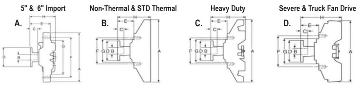
When disengaged, a fan clutch is designed to operate at 20 to 30 percent of the driven speed to help reduce the parasitic drain on the engine, increasing fuel economy. One of the primary differences between a Standard Duty, Heavy Duty, and Severe Duty fan clutch is the driven fan speed when engaged.
